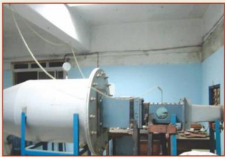
Supersonic Tunnel-Mach No: 2 (Test section size 15cm x 15cm x 30 cm)
