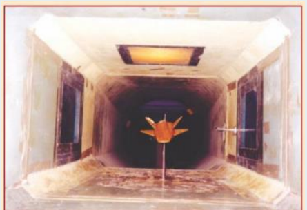
Subsonic Wind Tunnel Test Section (6' x 4' x 3', Max. wind speed 40 m/s)
