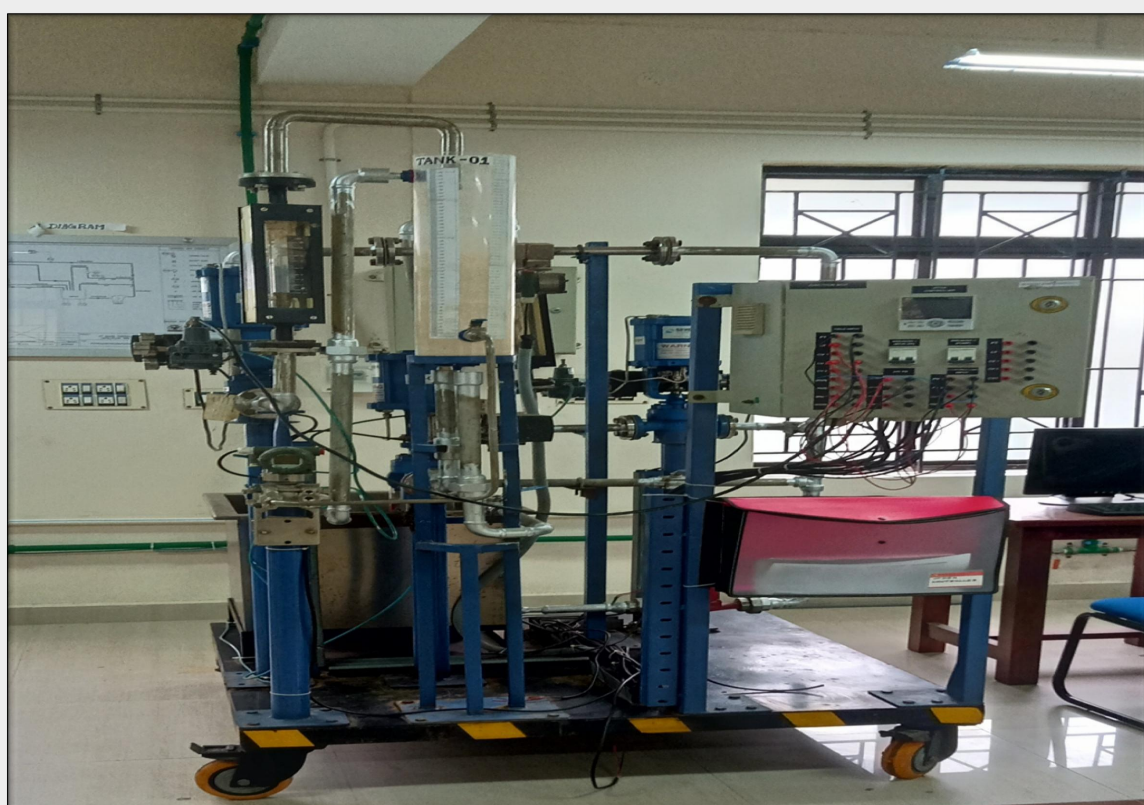
Level and Flow Control Station
