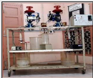
PH Control Test Rig
