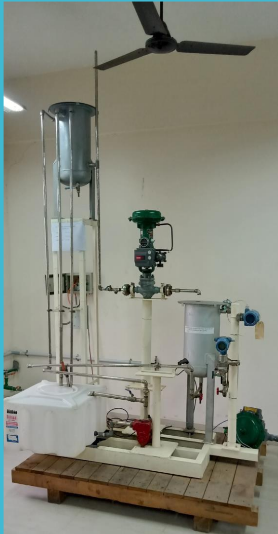
Reactor with Smart Field Devices
