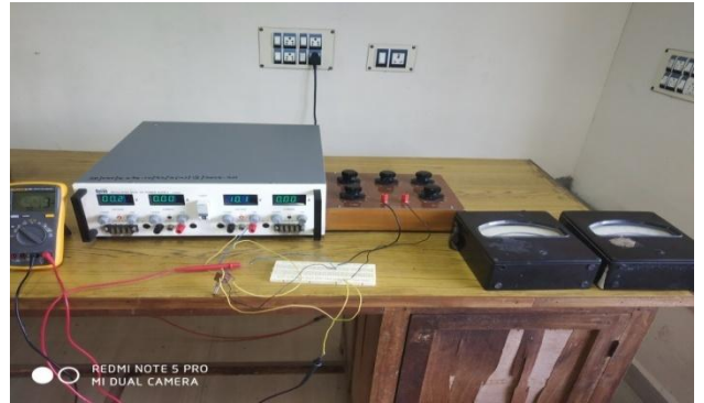
Anderson Bridge Experimental Setup
