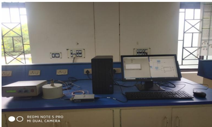
Schering Bridge Setup
