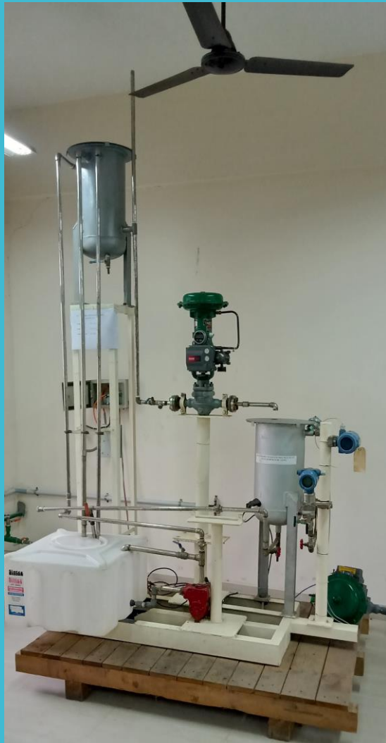
Reactor with Smart Field Devices
