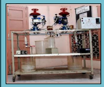
PH Control Test Rig
