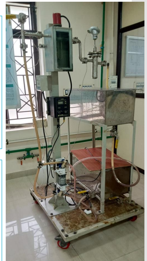
Temperature Control Process with Transportation Lag
