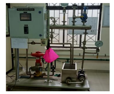
Pressure Control Process
