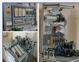
Servo Drive with Motor and Controller
